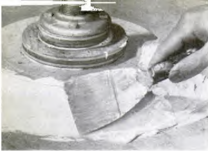
FIRST STEP in molding gracefully curved pedestal is to fill in "steps" using plaster of paris
